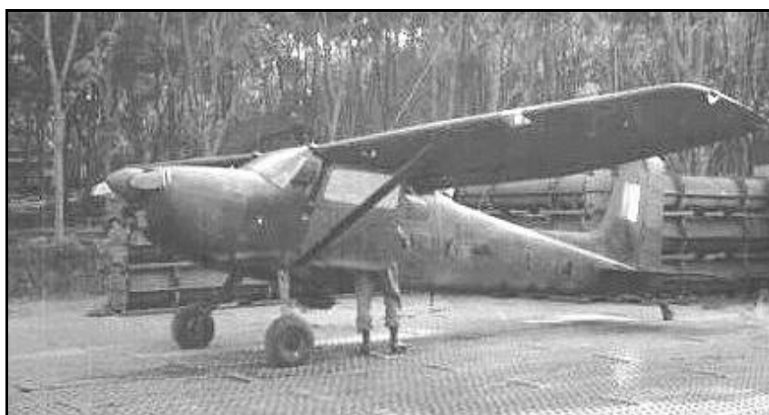
Above, one of the Cessna 180A aircraft used by 547 Signal Troop for ARDF missions.
